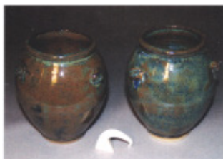
The same glaze can look different when applied on different clay bodies. Iron in the darker clay (left) reacted with the glaze and changed its color.
